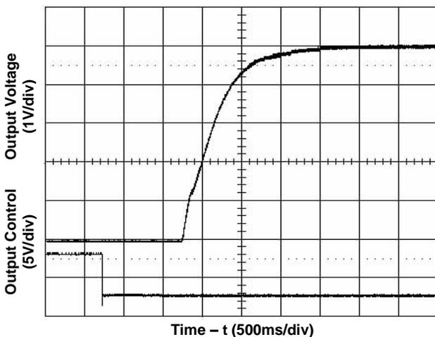
Figure 3. Start-Up from Enable Control
