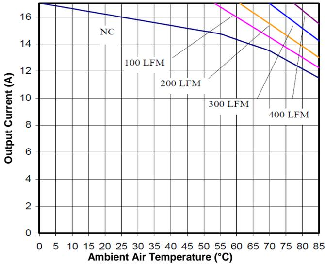
**Figure 11.** Current Derating Curve for Airflow Direction 3
