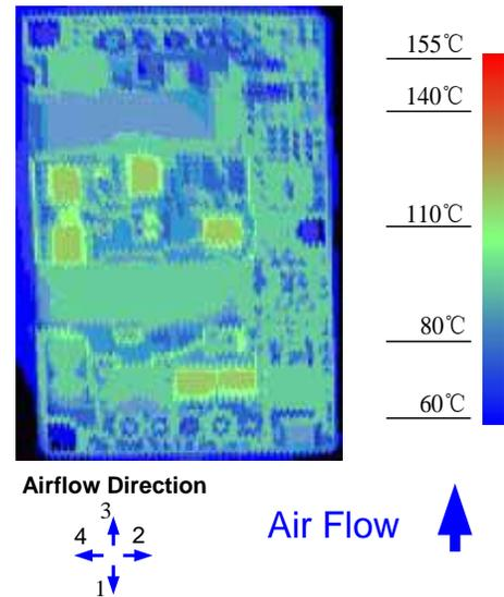
**Figure 14.** Thermal Image for Airflow Direction 4
