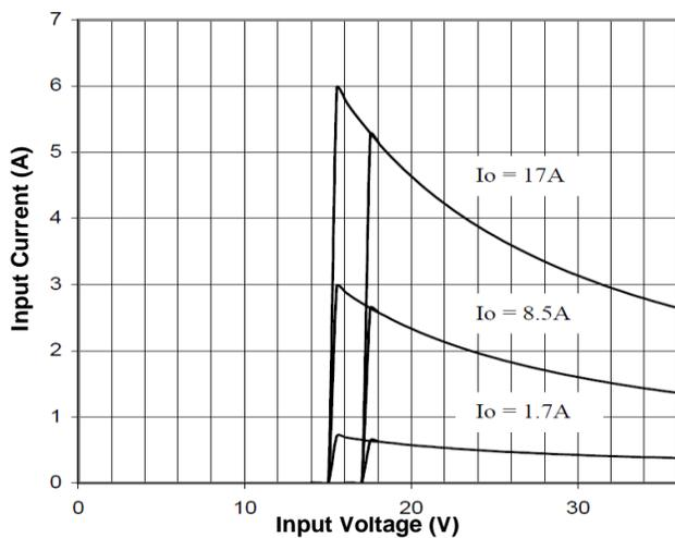
Figure 9. Input Characteristics
