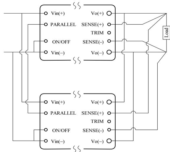
Fig. 20 Circuit Configuration for Active Current Share
