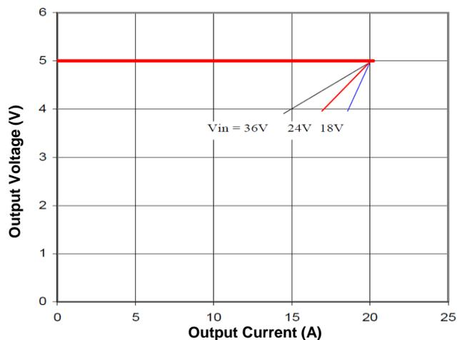
Figure 10. Output Characteristics
