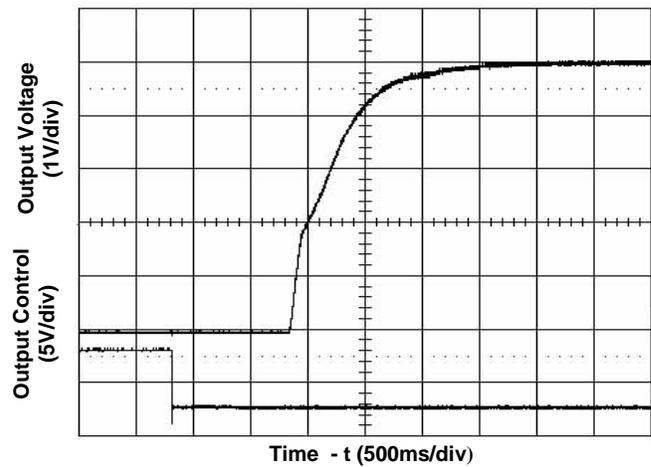
Figure 4. Start-Up from Enable Control
