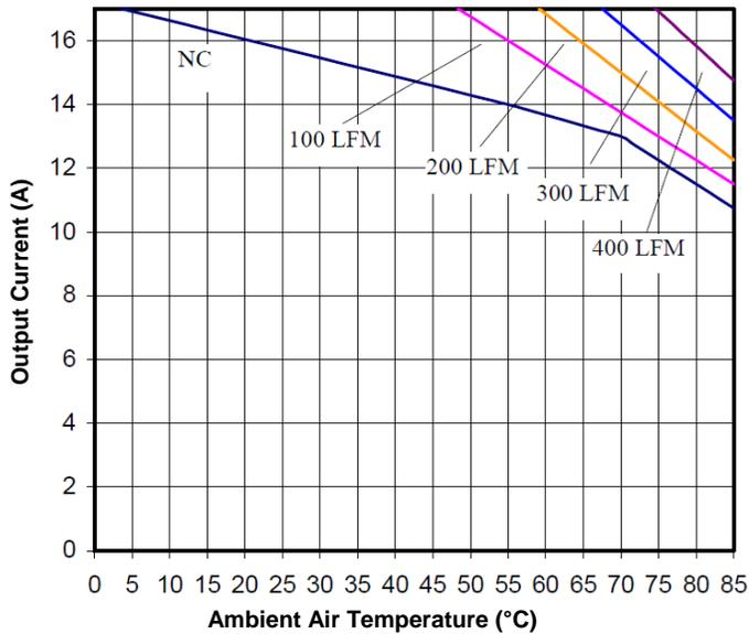
**Figure 13.** Current Derating Curve for Airflow Direction 4
