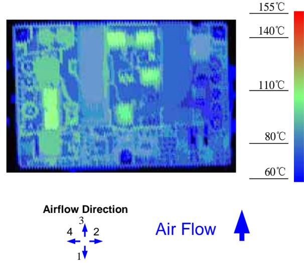
**Figure 12.** Thermal Image for Airflow Direction 3
