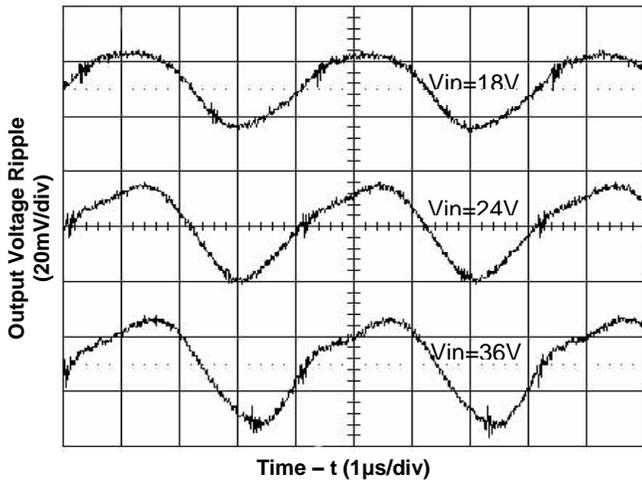
Figure 5. Output Ripple Voltage at Full Load
