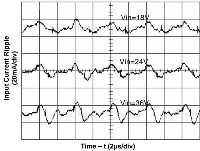
Figure 6. Input Reflected Ripple Current at Full Load
