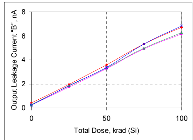
Figure 15. Output Leakage Current "B" vs Total Dose at V_F = 1.0 \text{ V} , V_{out} = 90 \text{ V} .
