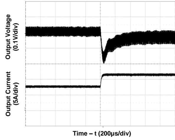
Figure 6. Transient Load Response
