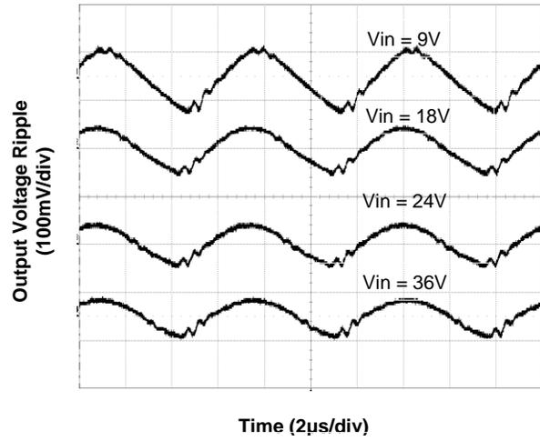
Figure 4. Output Ripple Voltage at Full Load
