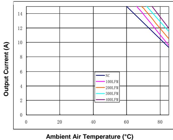
Figure 7. Current Derating Curve for Airflow Direction 1
