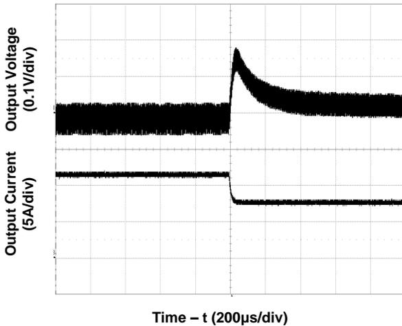
Figure 5. Transient Load Response
