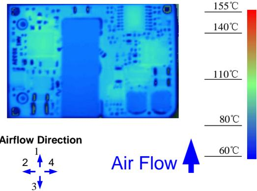
Figure 8. Thermal Image for Airflow Direction 1 (15A output, 55°C ambient, 200 LFM, typical Vin, open frame, unit soldered onto a fixture board.)
