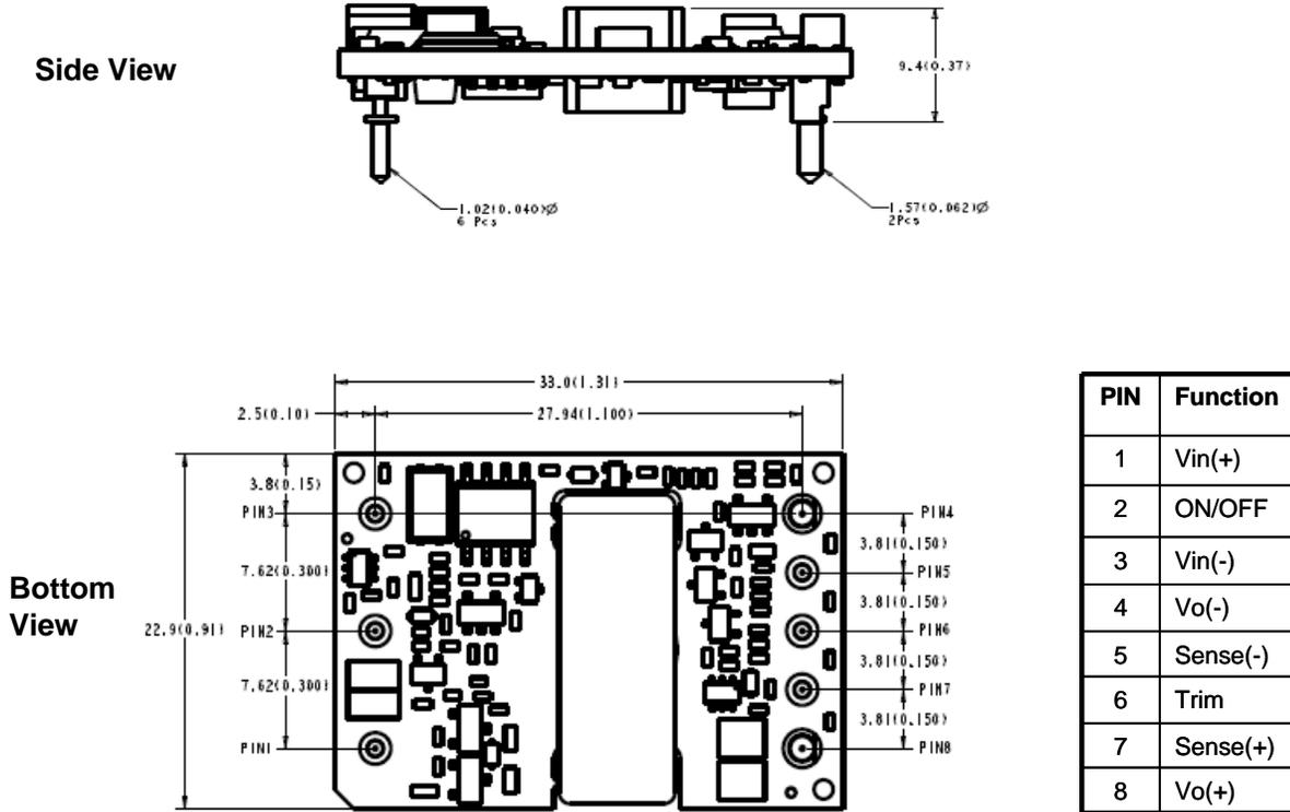
Figure 15. Open Frame Converter
