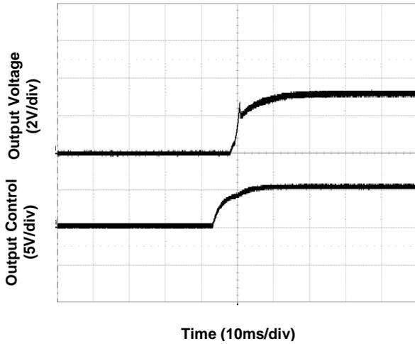
Figure 3. Start-Up from Enable Control
